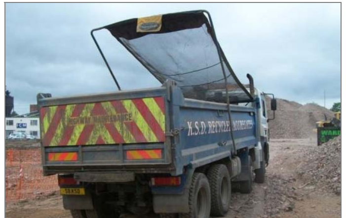
DISPOSAL OF RHIZOME CONTAMINATED SOILS BY REGISTERED CARRIER TO LICENSED DISPOSAL FACILITY
