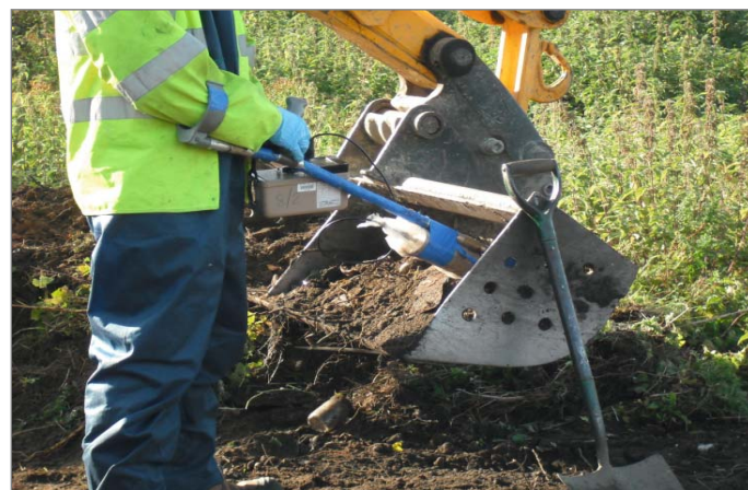
SCANNING EXCAVATED MATERIAL FOR SENTENCING
